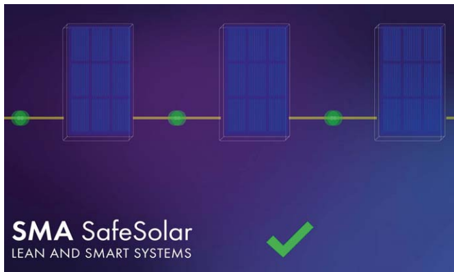
Diagram: The likelihood of cross-mating increases as the number of connectors in a PV system with MLPE increases. This can lead to dangerous electric arcs and can cause a PV system fire.
