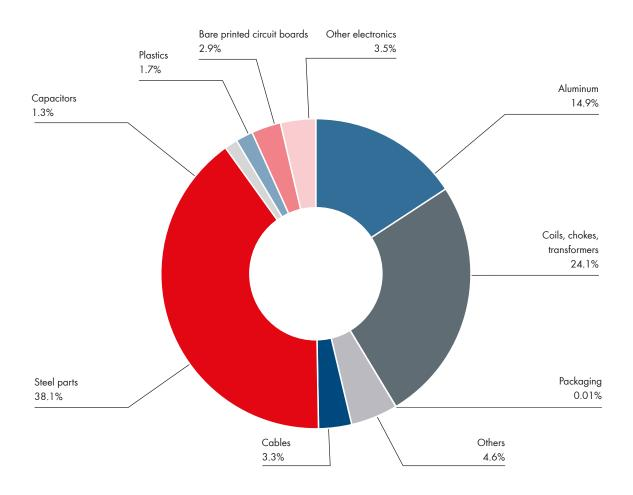
• Percentages of the total emissions of 14,037.8 kg CO2e per inverter caused by the individual materials and components used.
