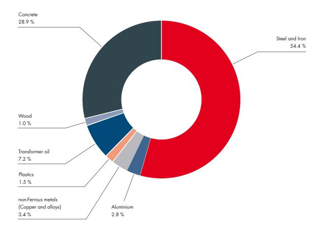
Percentage by mass of individual materials and components in an MVPS, total weight approximately 23.4 tonnes (including packaging and concrete foundation)
